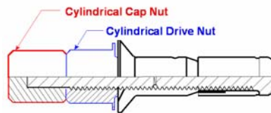
Left: A conceptual drawing of Monogram's Robotic Composi-Lok®
